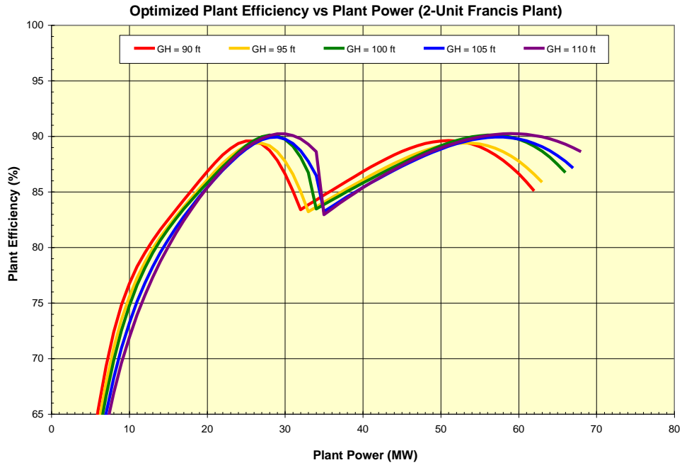
Figure 3-4: Optimized Plant Gross Head Efficiency versus Plant Power for Two-Unit Francis Plant
