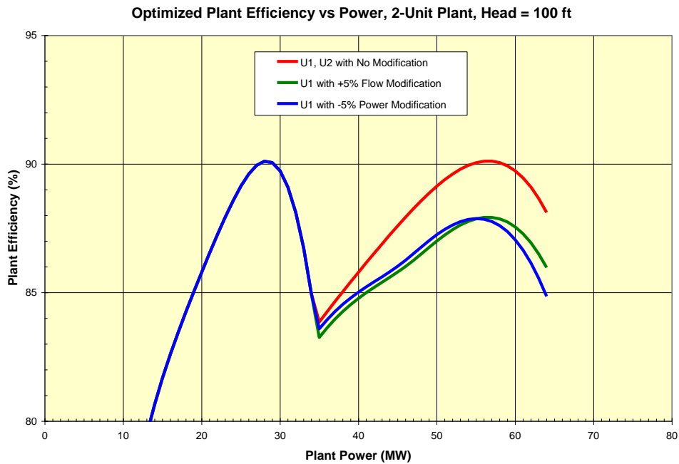
Figure 3-9: Optimized Plant Gross Head Efficiency versus Plant Power with Application of 5% Uncertainty to Flow and Power for Two-Unit Francis Plant
